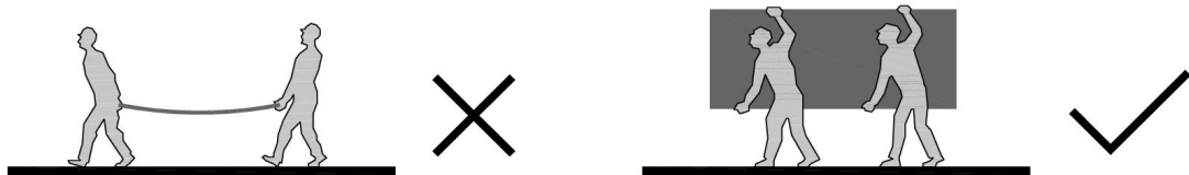
Figure 1.14 – Manutention des panneaux Viroc
